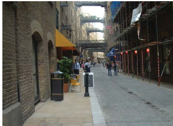
Contrasting materials between footways and carriageways
