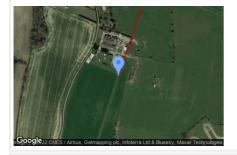
Name: Pent Farm RWY 05 Description: Threshold height : 15 m Direction: 51.0 deg Glide slope: 3.0 deg Pilot view restricted? Yes Vertical view restriction: 30.0 deg
