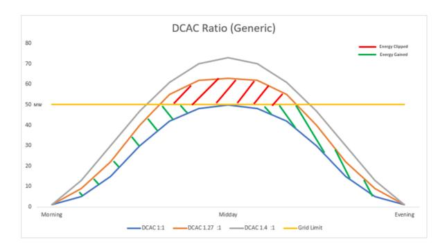
7. Distinct from this practice of generating station optimisation is what NPS EN3 defines as overplanting, which is a higher ratio that seeks to "take account of degradation in panel array efficiency over time, thereby enabling the grid connection to be maximised across the lifetime
